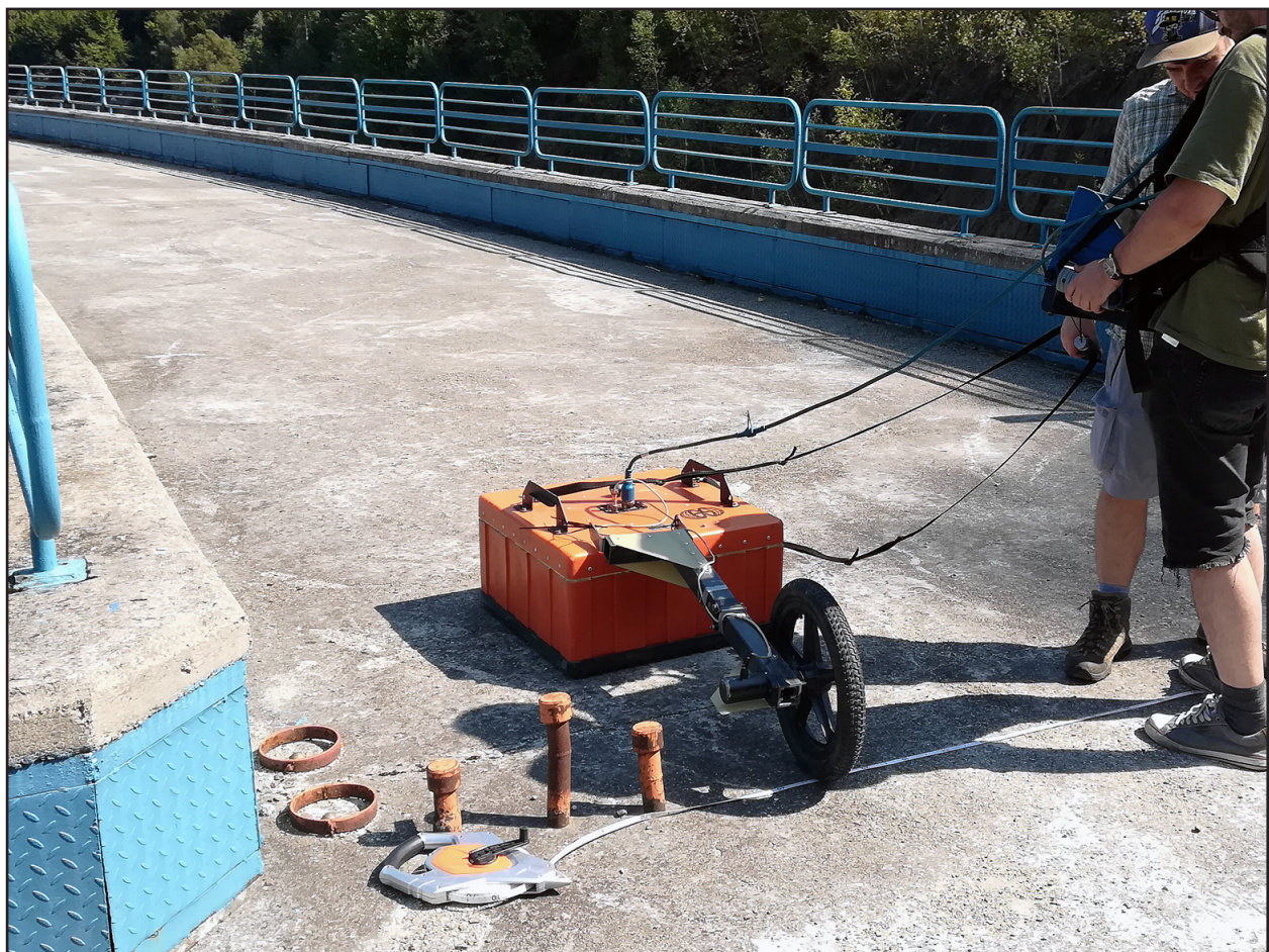
Fig. 4. The GPR equipment, formed of one 200 MHz antenna, a wheel for measuring distances and the GSSI-SIR 3000 console.
